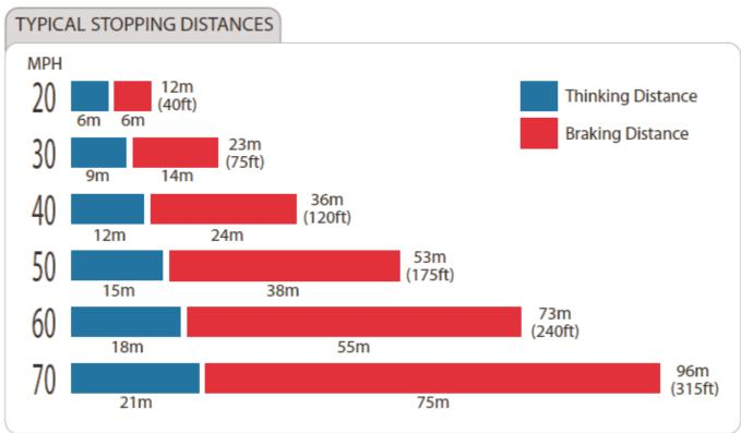
The Overall Stopping Distances are DOUBLED (x 2) for wet roads and multiplied by TEN (x 10) for snow and icy conditions.
